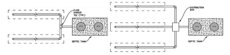
DEQ does not require installation of leach field trenches in a straight line. In fact, it is always preferable to follow the contour of the land. Additionally, never install the leach field in floodways, at the base of slopes, or in depressions where runoff water could flood the leach field. Construct leach fields in areas with good surface drainage, where the water cannot pond over the leach field.
