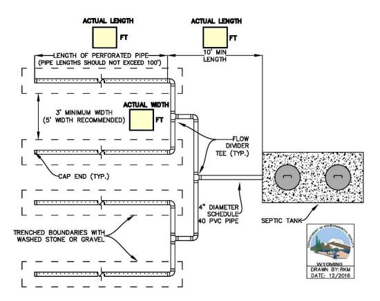
Draw your perforated pipe trench layout below or attach a separate sheet.
